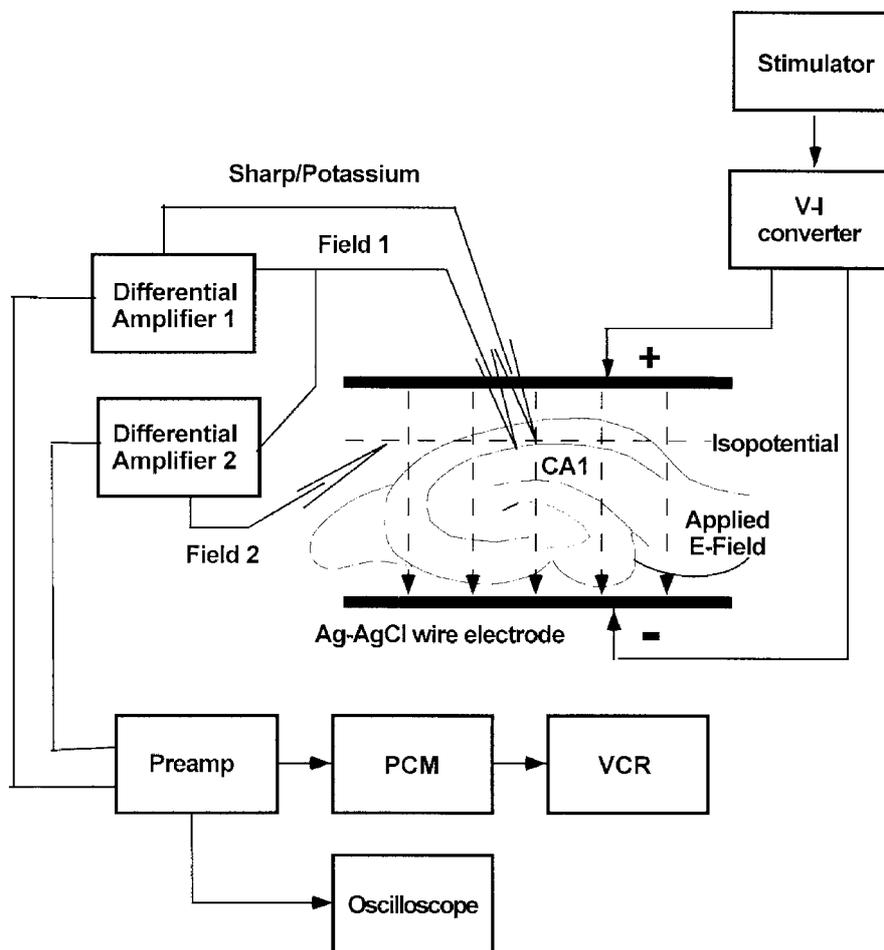
**Figure 1.** Experimental setup for application of uniform sinusoidal fields across hippocampal slices
